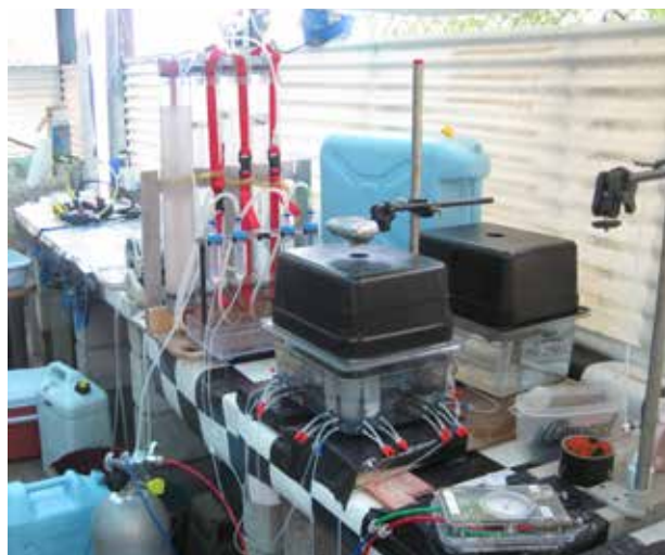
Figure 7. Design to test the navigational behavior of coral larvae to waterborne cues.
